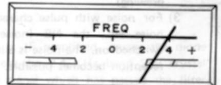
When the center meter swings to the right, the frequency of the opposite station is higher than receiving frequency.
