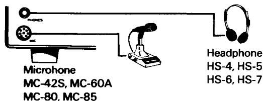
Either a low or high impedance microphone ( $500 \Omega \sim 50 \text{ k}\Omega$ ) may be used. The PTT switch must be isolated from the microphone audio circuit, as shown in **A**. Use a mi-
