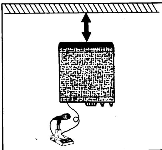
Allow at least 3 inches clearance between the back of the equipment to any object. This space allows an adequate airflow from the ventilating fans to keep the transceiver cool.
